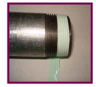
Hold tape taut while wrapping, to insure tape molds into root of threads.
