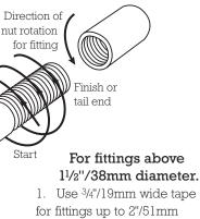
for fittings up to 2"/51mm diameter. Use 1" wide tape for fittings larger than 2"/51mm diameter.
